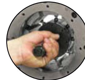
Quick Change Tool Makes die changes a quick and simple process.
